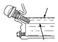
Figure 5. Engine Oil Dipstick (Oil Level)
